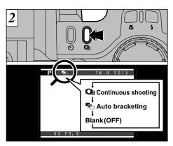
After selecting AUTO BRACKETING, press the "" button so that the "" icon appears on the screen. The mode switches (" • " • Blank) each time you press the "" button.
